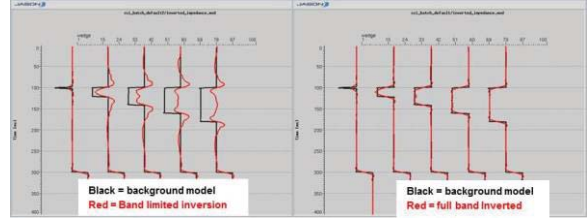
Figure 4: Cross sections illustrate the side lobe effects (left) on inverted results when low frequencies are missing in inversion. The picture on the right shows side lobes are removed if the correct low-frequency model is included in inversion.
